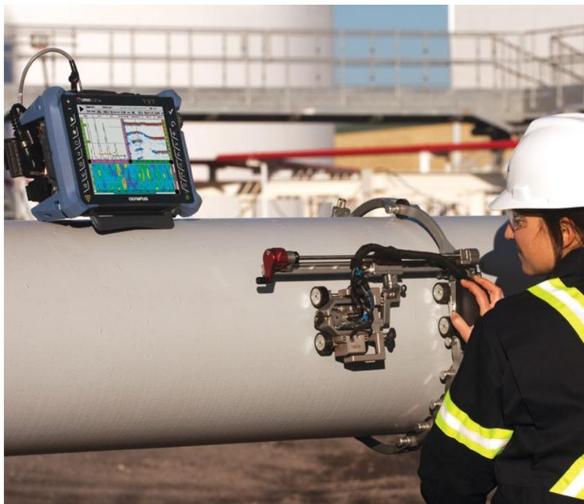
The HydroFORM and RexoFORM scanners are designed to offer the best inspection solution for the detection of wall-thickness reductions due to corrosion, abrasion, and erosion. Our solution also detects mid-wall damage such as hydrogen-induced blistering or manufacturing-induced laminations and easily differentiates these anomalies from loss of wall thickness.
