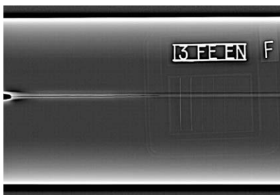
Thin-walled stainless steel cylinder with longitudinal weld seam.
