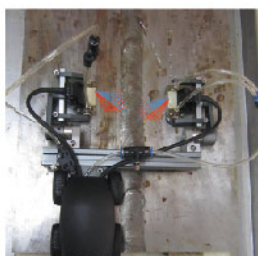
Dual-side Butt Weld Inspection
