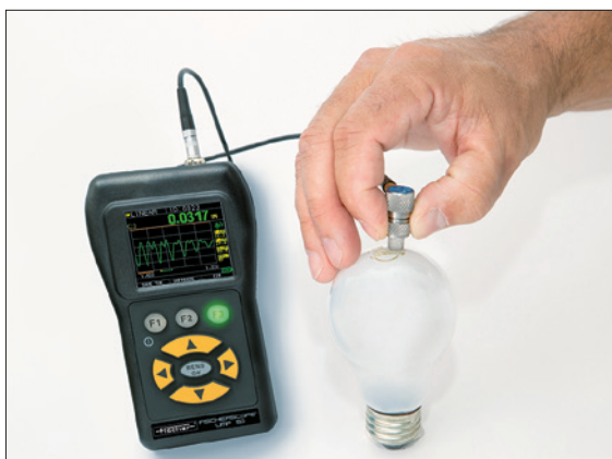
Vibrating alarm and colored LEDs indicate when a threshold has been violated
